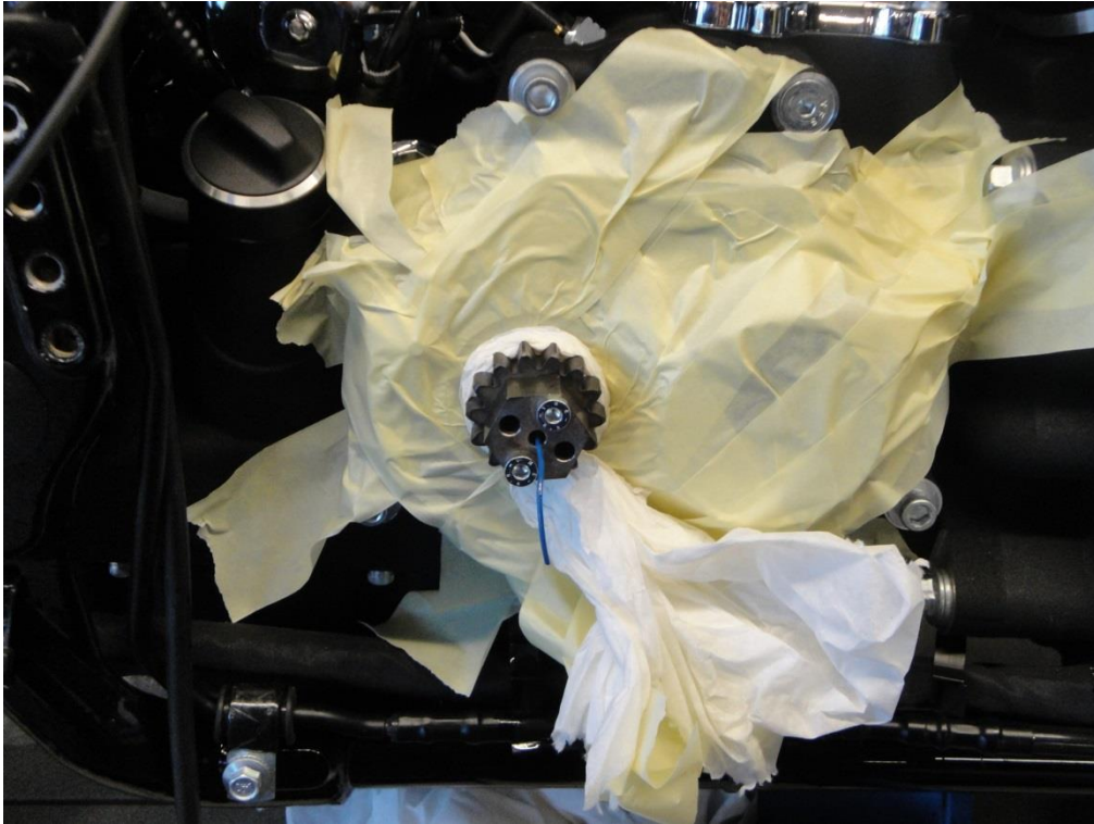
Use masking tape to mask the gearbox. So no steel shivers can come into the gearbox!
