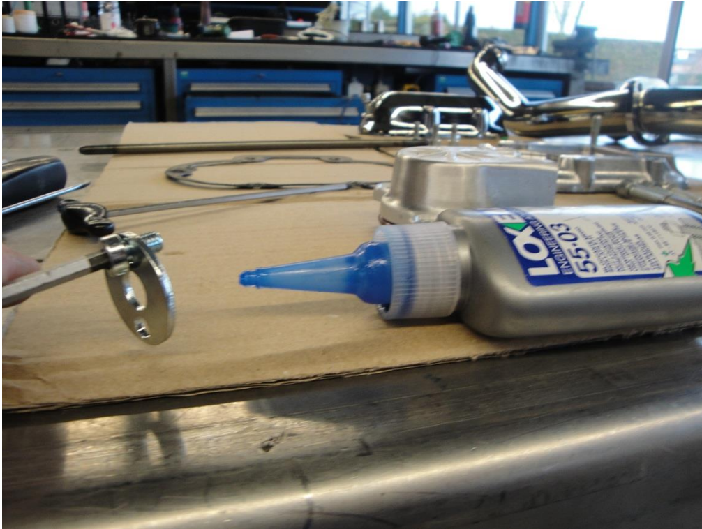
Mount the plate with some (normal) Loctite.
