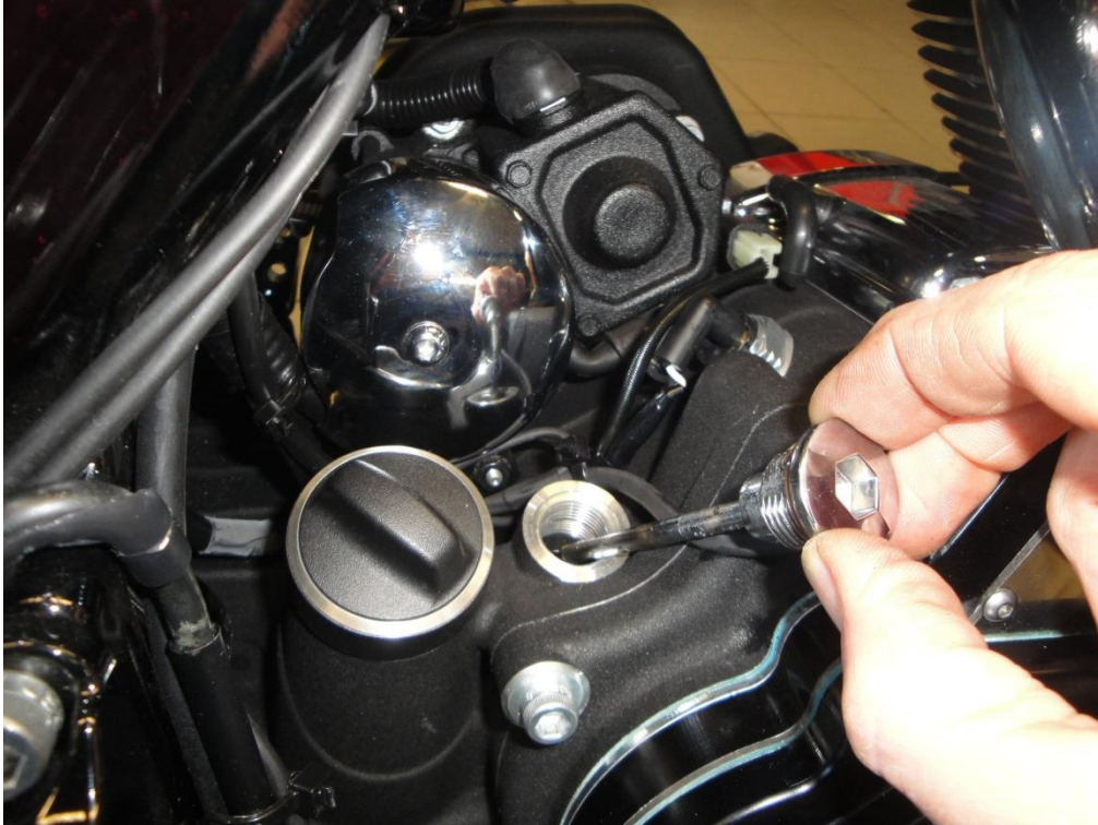
Check the level of the gearbox oil.
