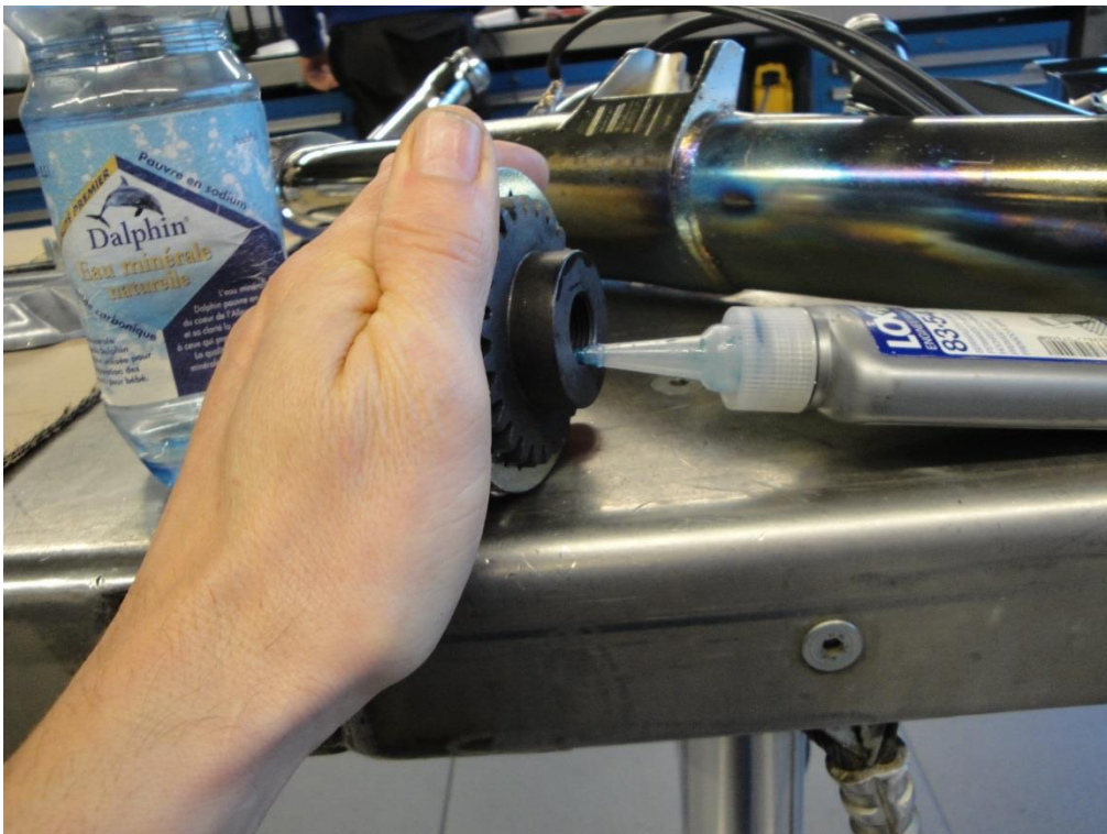
Mount the sprocket with strong Loctite.
