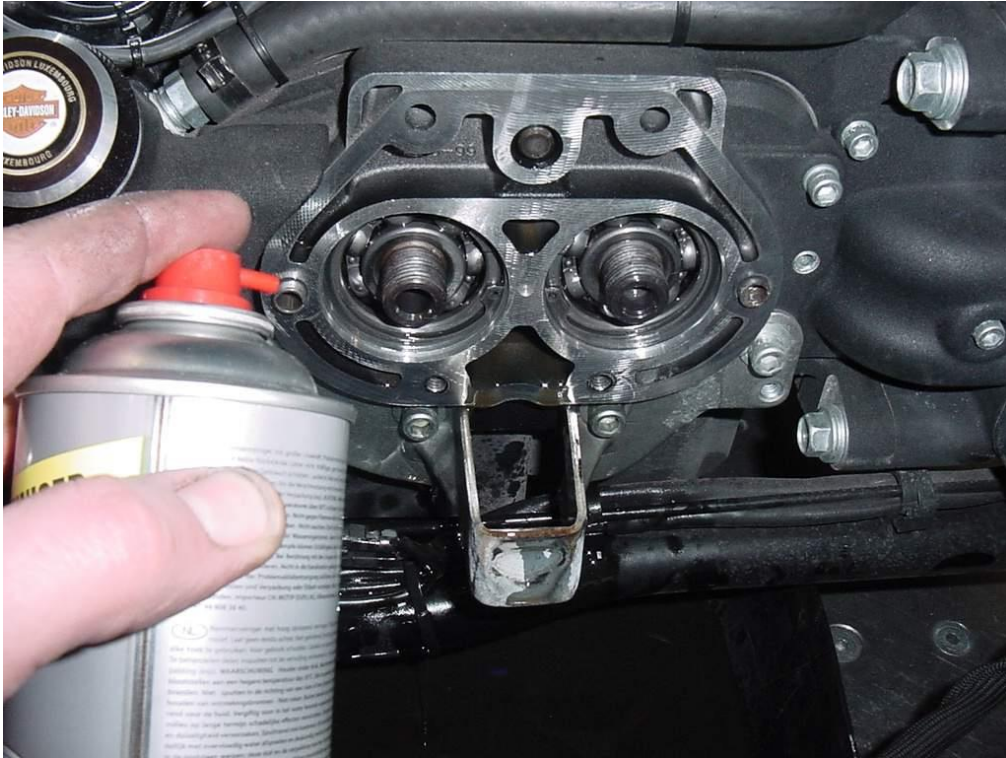
Clean the screw-thread with brake cleaner.
