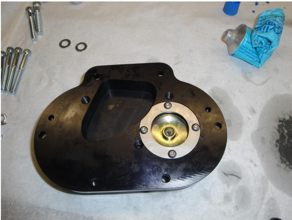
Mount the piston in the EML housing using some (normal) Loctite.
